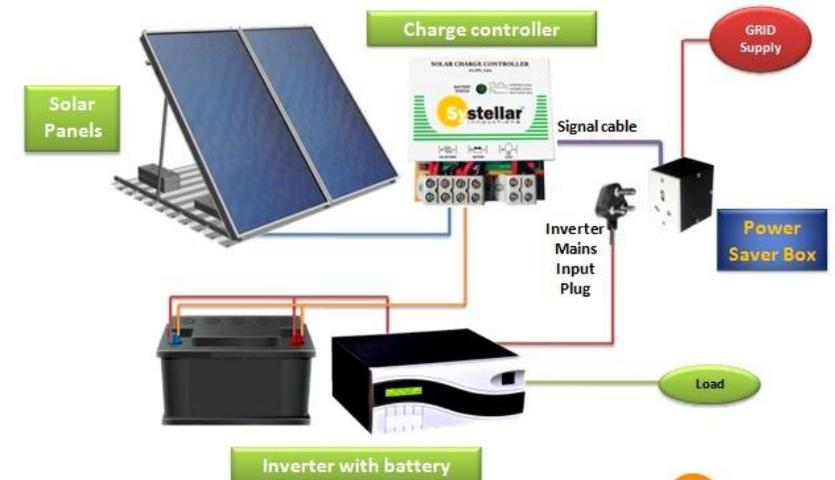
Inverter Mains Input Plug needs to be inserted into Power Saver Box
